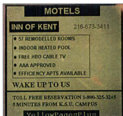
Figure 1 A bistable reflective mode 320 x 320 telephone display prototype using polymer stabilized cholesteric texture (PSCT) technology. The display, developed at the NSF Center ALCOM at Kent State University, is shown removed from its drive circuitry to illustrate its bistable memory.
